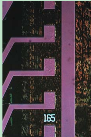
LCD circuit(60X coaxial illumination observing)
