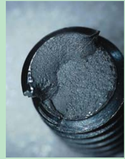
Bolt's section (30X observing)
